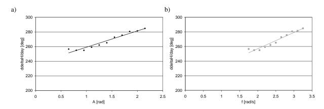
Fig. 7. "Avoidance of an obstacle having suddenly sprung up." Range of values of the factor  $\frac{d\delta_H}{da_y}$  depending on: a) Steering wheel input amplitude A; b) Steering input frequency f
