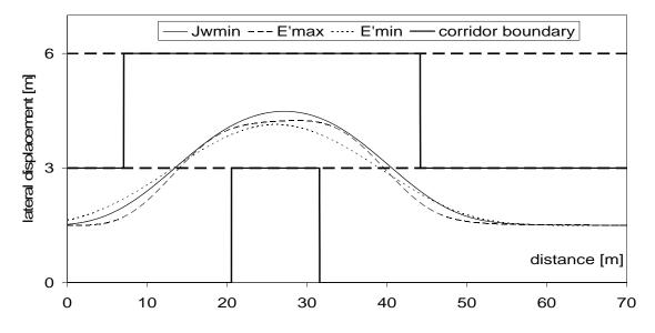
Fig. 3. Vehicle trajectory at the manoeuvre "avoidance of an obstacle having suddenly sprung up"
