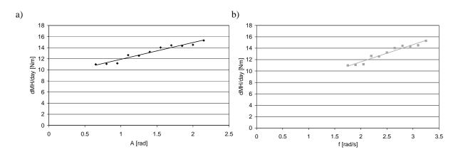
Fig. 6. "Avoidance of an obstacle having suddenly sprung up." Range of values of the factor  $\frac{dM_H}{da_y}$  depending on: a) Steering wheel input amplitude A; b) Steering input frequency f
