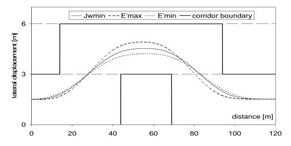
Fig. 4. Vehicle trajectory at the manoeuvre "avoidance of an obstacle without the element of surprise"
