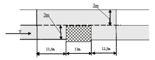
Fig. 1. Corridor for the manoeuvre "avoidance of an obstacle having suddenly sprung up"
