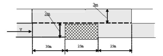
Fig. 2. Corridor for the manoeuvre "avoidance of an obstacle without the element of surprise"
