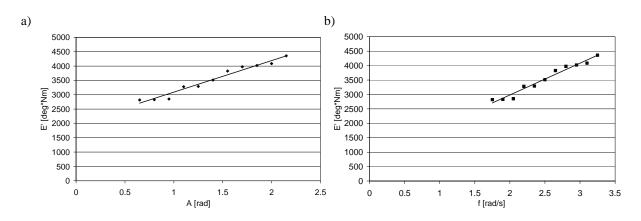
*Fig. 5. "Avoidance of an obstacle having suddenly sprung up." Range of values of the steering effort E' depending on: a) steering wheel input amplitude A; b) steering input frequency f*
