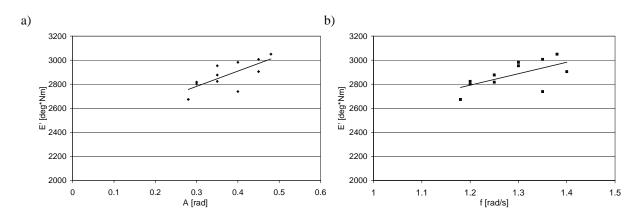
*Fig. 8. "Avoidance of an obstacle without the element of surprise." Range of values of the steering effort E' depending on: a) Steering wheel input amplitude A; b) Steering input frequency f*
