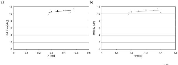
Fig. 9. "Avoidance of an obstacle without the element of surprise." Range of values of the factor  $\frac{dM_H}{da_y}$  depending on: a) Steering wheel input amplitude A; b) Steering input frequency f
